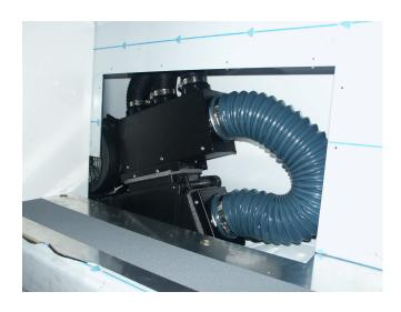
After Aluminum insert is installed and tested, attach cover plate to bench / wall to cover OEM Rear AC/Heat Unit using #10 Sheet metal screws.
